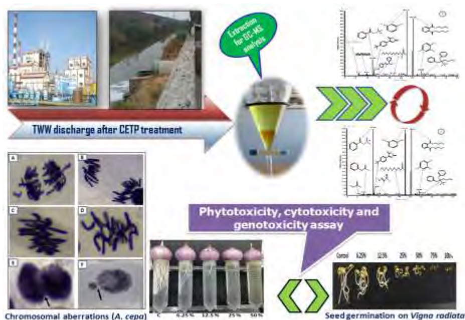
Schematic presentation for detection of pollutants in tannery waste water and their toxicity
