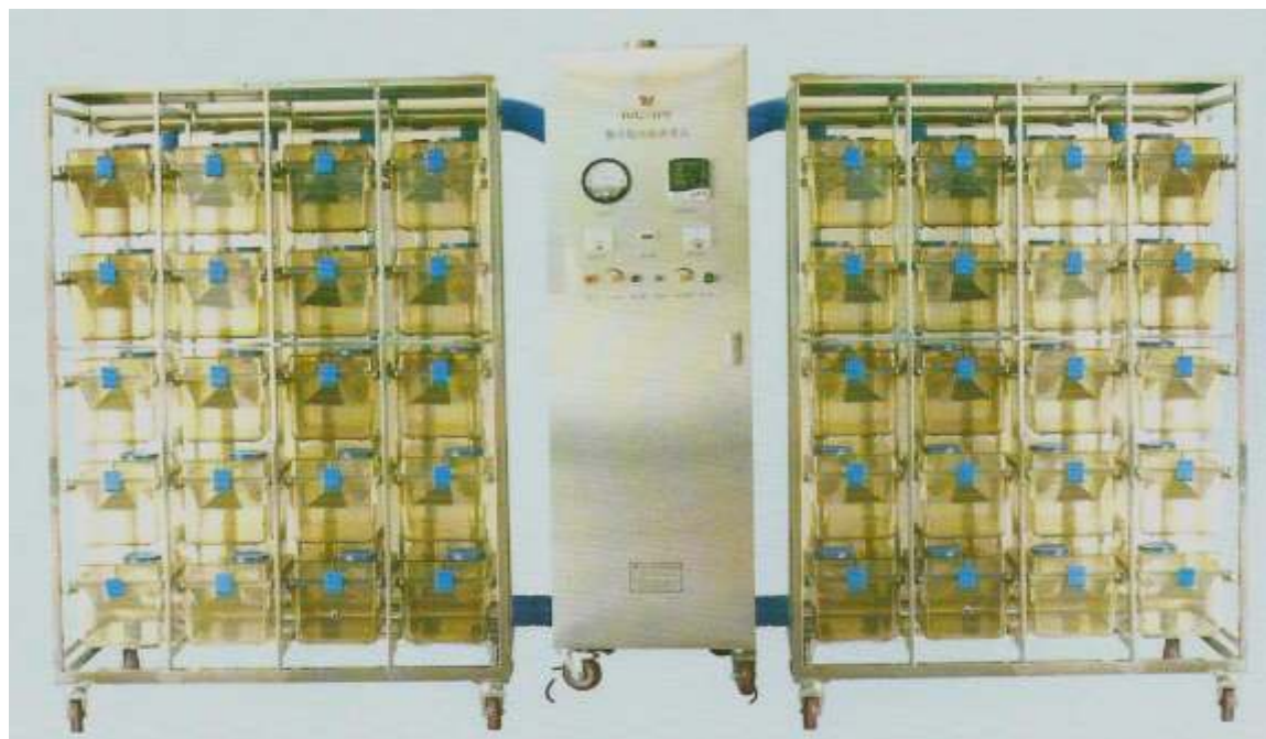
Individually ventilated cage system
